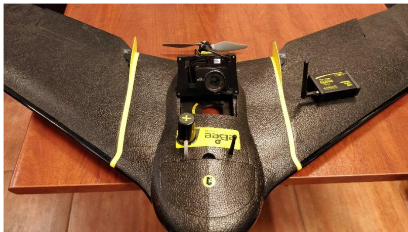
Figure 1. SenseFly's eBee, the RGB camera and the antenna
